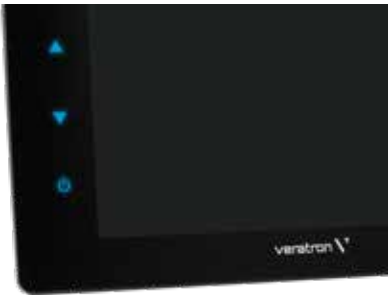
Lateral touch buttons are RGB illuminated and allow for a quick brightness adjustment
