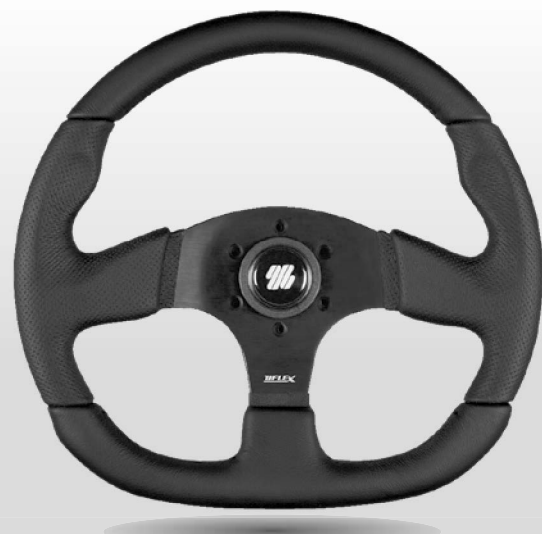
Palmaria B/B 63727H 350 mm (13.8") Depth 40 mm (1.57") Black polyurethane grip, black aluminium spokes
