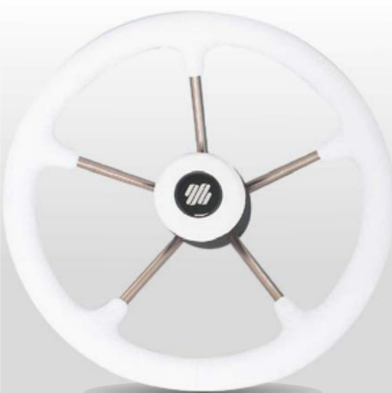
V70W 39929J 350 mm (13.8") Depth 90 mm (3.54") White polyurethane grip, SS spokes
