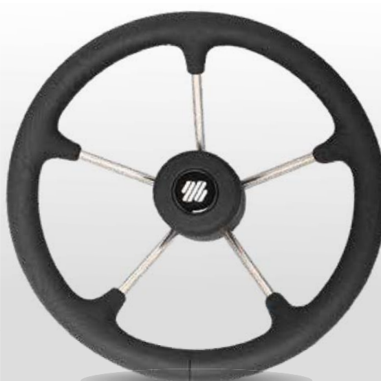
V70B 39442D 350 mm (13.8") Depth 90 mm (3.54") Black polyurethane grip, SS spokes
