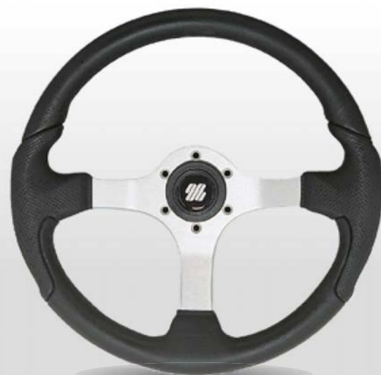
Nisida B/S 61813P 350 mm (13.8") Depth 85 mm (3.35") Black polyurethane grip, silver aluminium spokes
