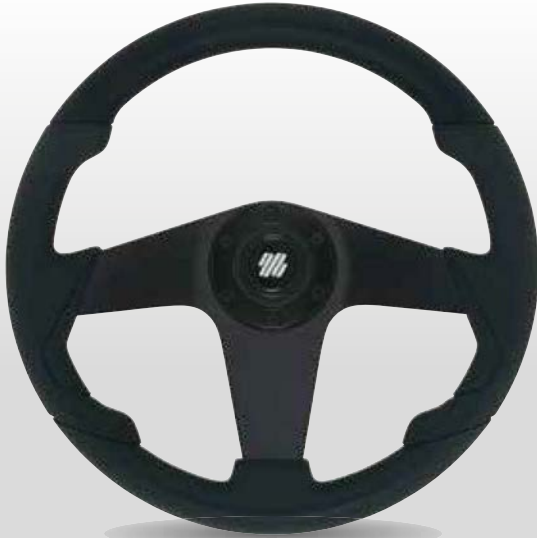
Pianosa B/B 22960H 350 mm (13.8") Depth 88 mm (3.46") Black polyurethane grip, black aluminium spokes, black painted ring
