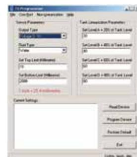
BEP Marine's proprietary software allows distributors or volume users to pre-programme tank dimensions giving accurate measurement avoiding experimental tank filling
