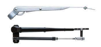
Note: pantographic wiper arms will ONLY function properly with wiper motor sweep angles 80° or less
