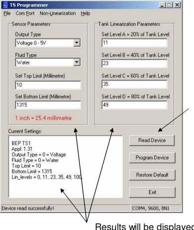
Press the **Read Device** button to retrieve the firmware version and parameter values from the TS1.
