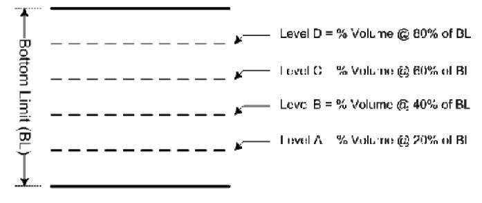
\* Tank's bottom limit is a user setting and can be different from tank's depth or height!
